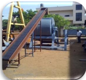
Rotary Dryer / Chillies & Turmeric
